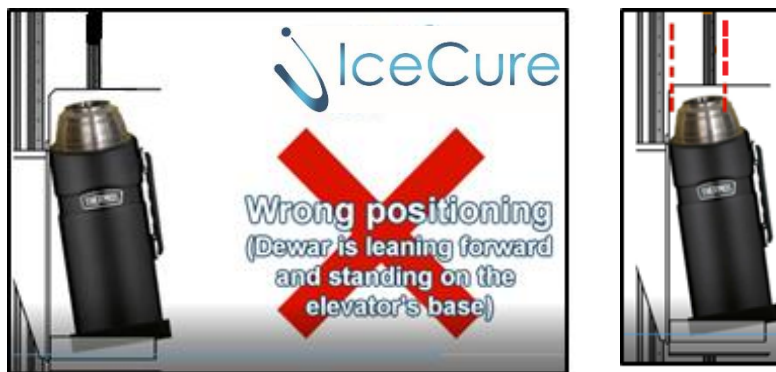
Figure 35: Insertion of the Dewar – head first, leaning forward
