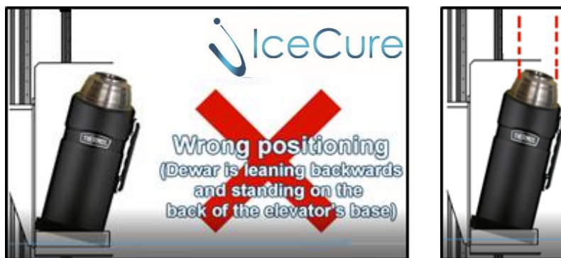
Figure 36: Insertion of the Dewar - bottom first, leaning backwards
