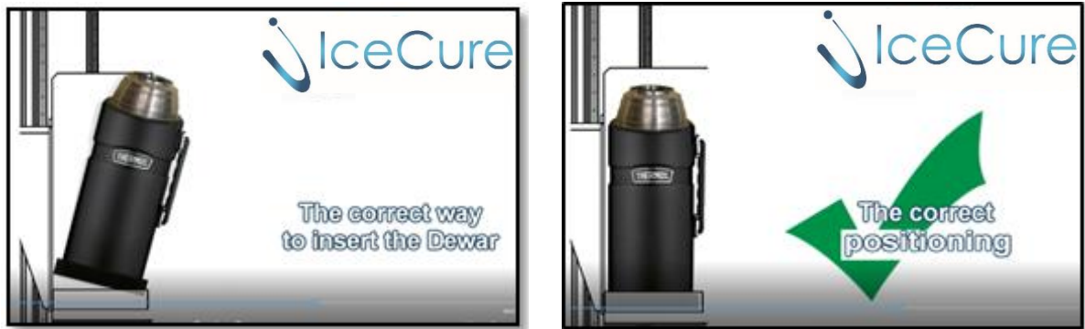
Figure 34: Correct insertion and positioning of the Dewar – bottom first
