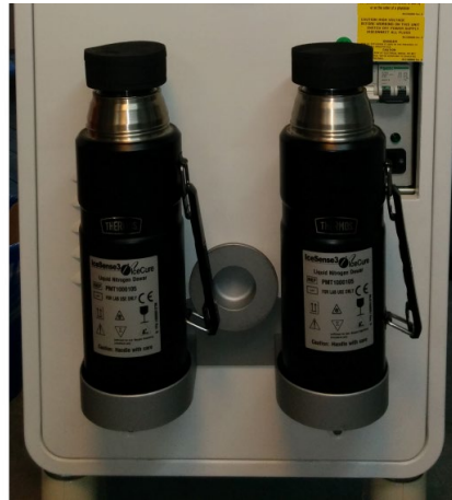
Figure 13: Dewar storage cases – the correct way to put the Dewars inside the storage shelf.
