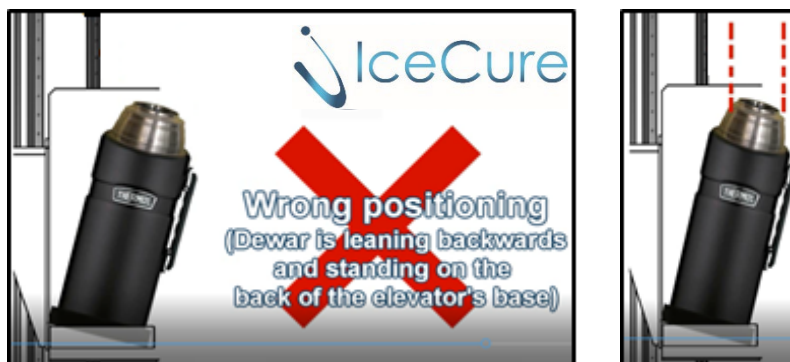
Figure 31: Insertion of the Dewar - bottom first, leaning backwards
