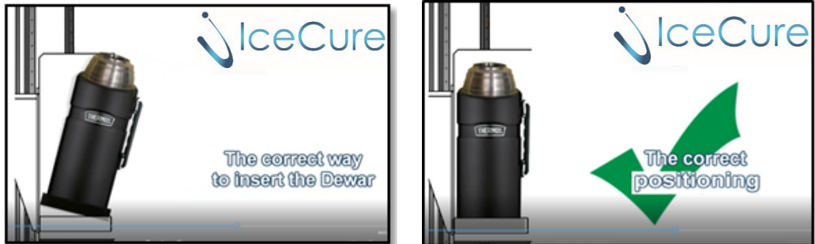
Figure 29: Correct insertion and positioning of the Dewar – bottom first
