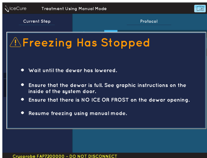
Figure 80: Replacement during Freeze, in case of empty Dewar.
