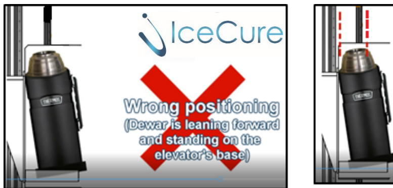
Figure 30: Insertion of the Dewar – head first, leaning forward
