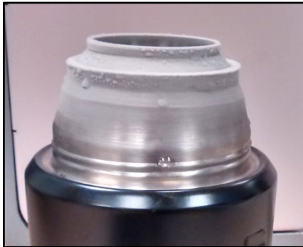
Figure 27: Frost on the Dewar opening
